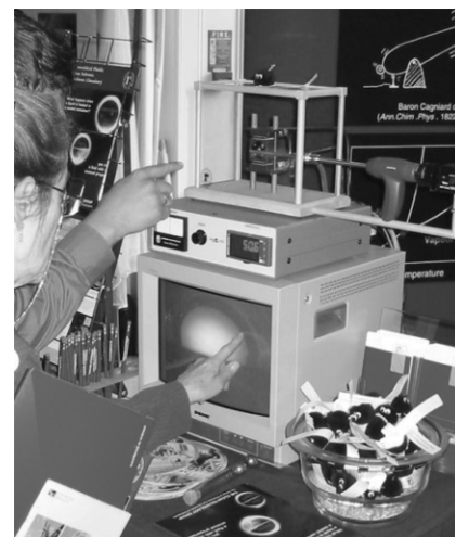
Fig. 5 Interactive critical point demonstration. N.B. the supporting laboratory recirculation bath is positioned under the surface of the table.
